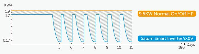
Saturn Smart Inverter HP VS Normal On/Off HP (Heating capacity 9.5kW)
