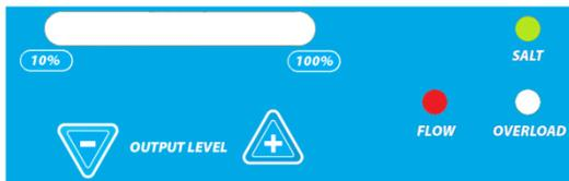
Flow Fault detected.
