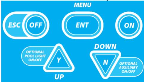
Each button is labelled with its primary function either on the button itself, or adjacent to it. Secondary functions are labelled within a curved white outline next to the relevant button.
