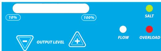
Overload detected, Cell has been turned off.
